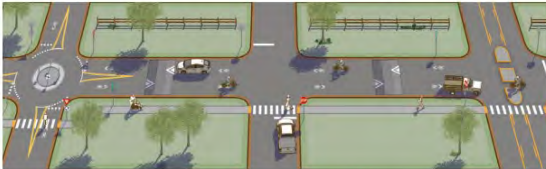
Figure 2-5. Bicycle boulevards combine road markings, traffic-calming measures, and crossing improvements designed to enhance the comfort and priority of bicyclists traveling along the route.
